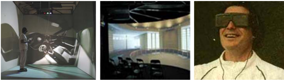
Figure 2. Projection based immersive VR system : CAVE :Cave Automatic Virtual Environment(left), Curved Wall (middle), 3D Stereo glasses(right)
